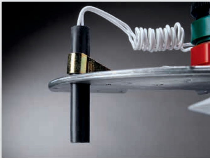
HEATER: A self-regulating heater can be added to prevent possible damage to electrical components due to condensation build-up inside the actuator. Mounted in the actuator top plate for easy accessibility.
